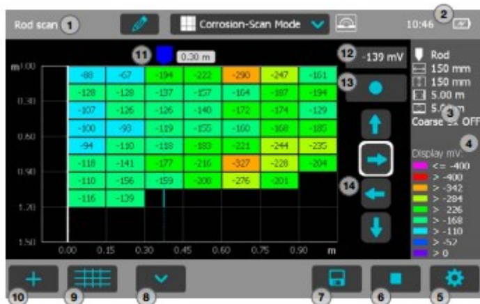
Figure 36: Corrosion-Scan Mode with rod electrode
