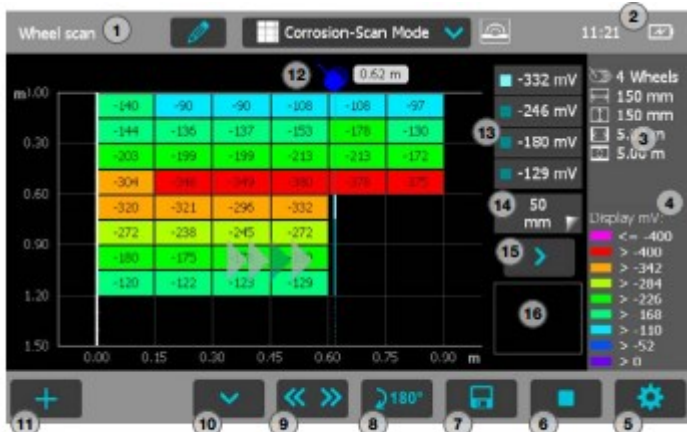
Figure 37: Corrosion-Scan Mode with one and four wheel electrode
